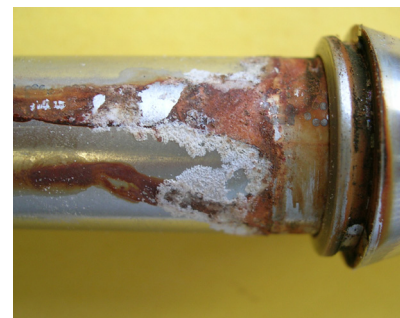
Picture of a low cost product. Corrosion damage created by a low quality hardening process applied to the back ferrule
